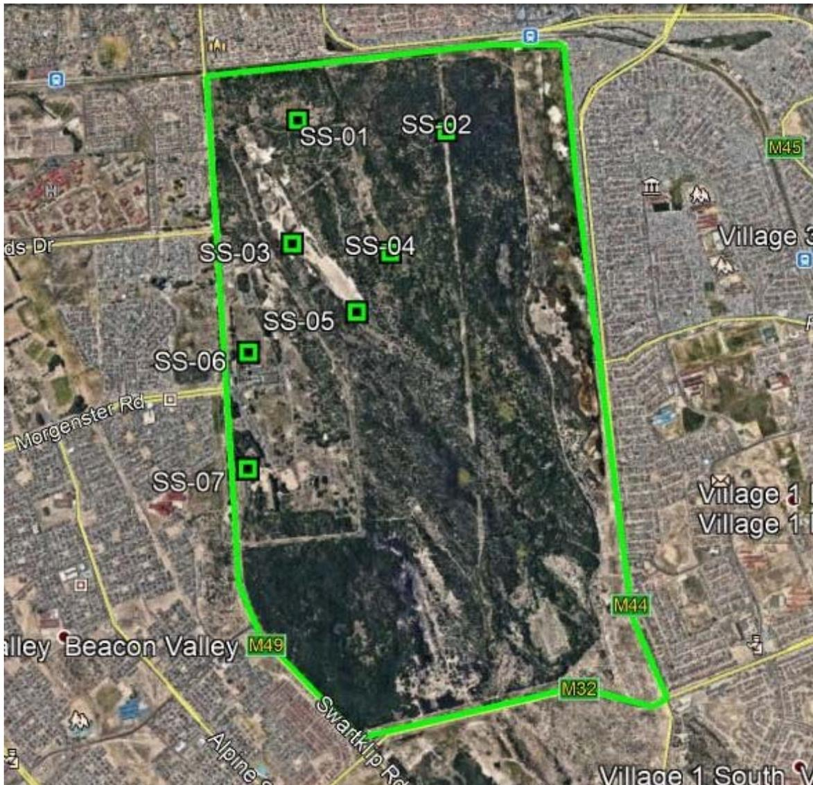
**Figure 3: Additional Soil Sampling Locations (courtesy of Google Earth)**
